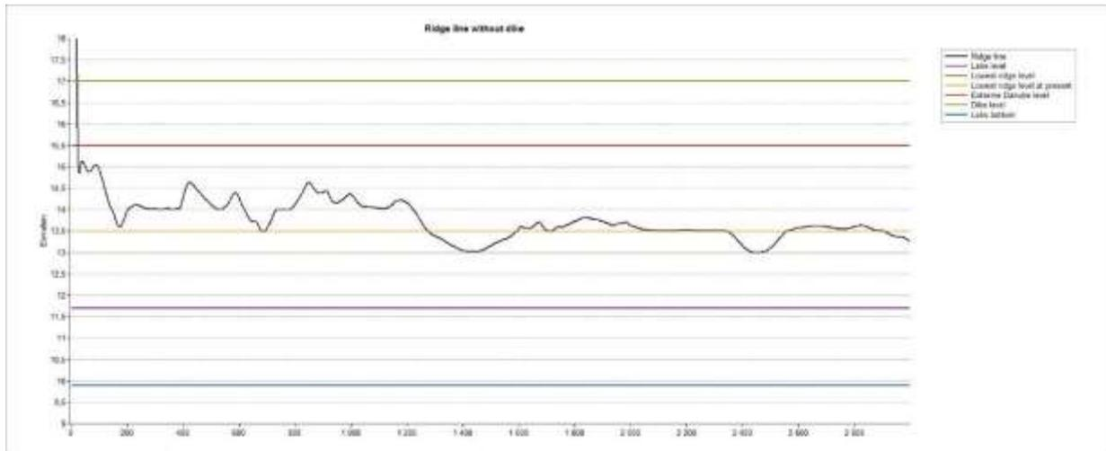
*Ridge profile between Lake Srebarna and the Danube. At present, the connection between the Danube and Srebarna is through the stretch from 0 m to 800 m (a stretch of breached dike), theoretically at levels above 13.50 m a.s.l. (in practice at levels above 14.00 m a.s.l.).*
